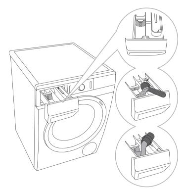
A separator/divider tab is supplied with the washing machine, which allows adding liquid detergent to the main wash compartment (left compartment).
