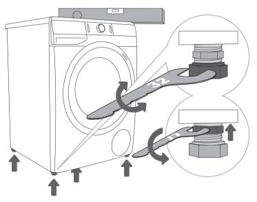
Level the washing machine in longitudinal and traverse direction by rotating the adjustable feet.
