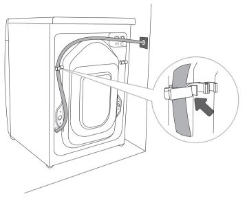
**D** The discharge hose has to be attached and affixed to the pin on the back of the washing machine, as shown in the figure.
