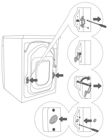
Move the hoses and undo the screws on the back of the washing machine. Remove the two angular pieces.
