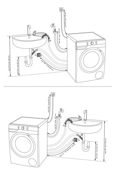
A Discharge hose end may be placed over a washbasin or a bathtub. B Use a string fed through the opening in the elbow support to attach the hose and prevent it from slipping to the floor.
