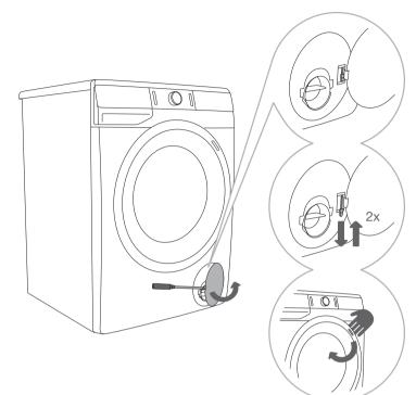
When the program is paused or interrupted, open the filter cap using a suitable tool (flat screwdriver or a similar tool).
