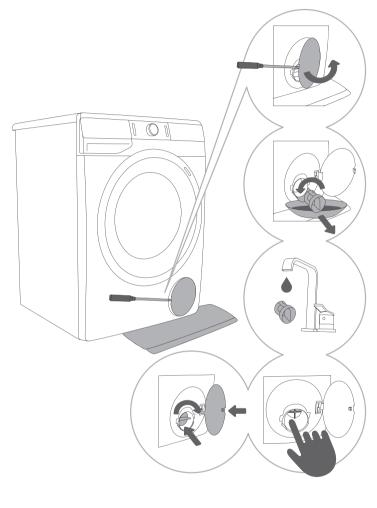
• Open the pump filter cap using a suitable tool (flat screwdriver or a similar tool).
