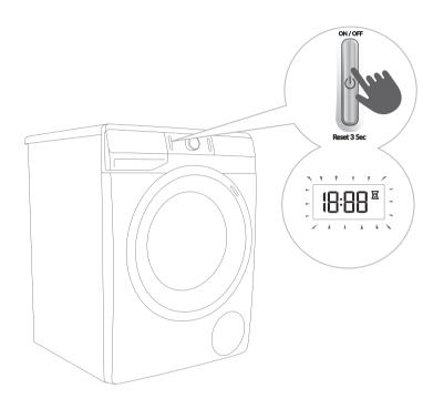
**To stop and cancel a washing programme,** press the (1) ON/OFF/**Reset** button and hold it for more than 3 seconds.
